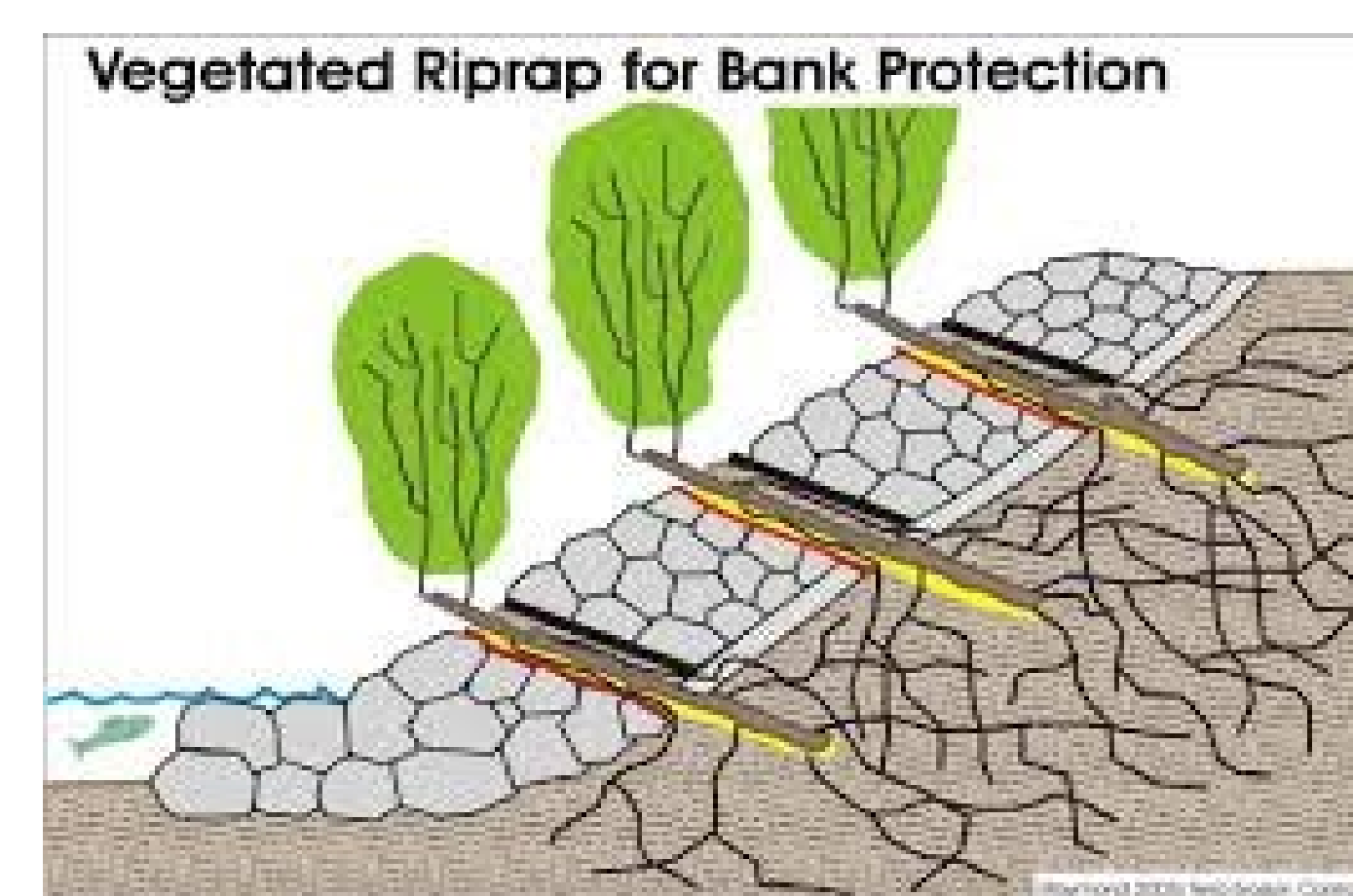
Figure 4: Vegetative riprap cross section 11
