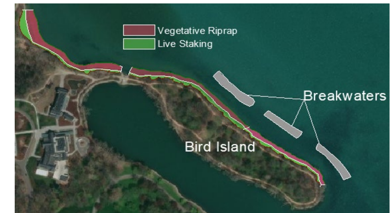
Figure 5: Proposed breakwater and shoreline design aerial view
